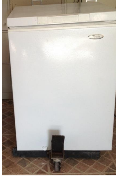
Figure 3.5 The testing unit is a 5 ft 3 Whirlpool refrigerator/freezer. It was placed in a controlled environmental chamber where the ambient temperature, air pressure and humidity were controlled based on ASHRAE testing standards.
